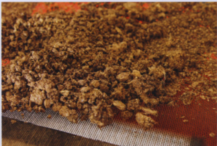
Before the pyrolysis process can begin, the poultry litter needs to be reduced from about 25 percent moisture content to 10 percent.
