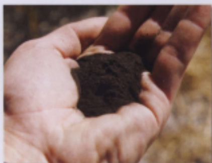
The char powder left after the pyrolysis process is completed is separated, stabilized and placed into barrels or bags. It is intended for use as fertilizer, boasting proportions of 4-4-5.
